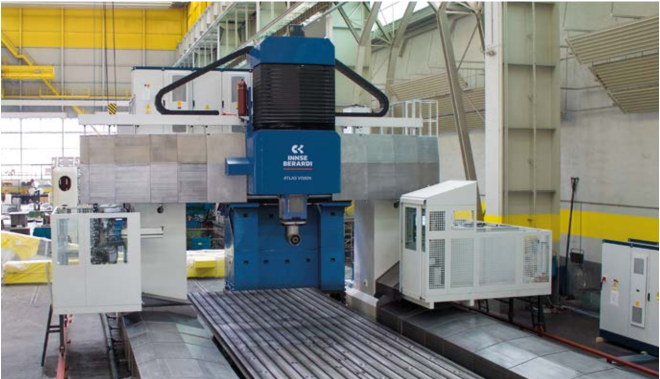
G: Gantry type - lower rails
