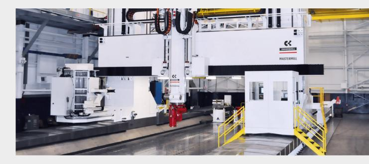
Ingersoll MasterMill builds on the worldwide successes of several generations of Ingersoll gantry-type equipment. MasterMill incorporates the latest finite element analysis designs to optimize the highly rigid machine structure, and new technology features to maximize machine performance and safety:
